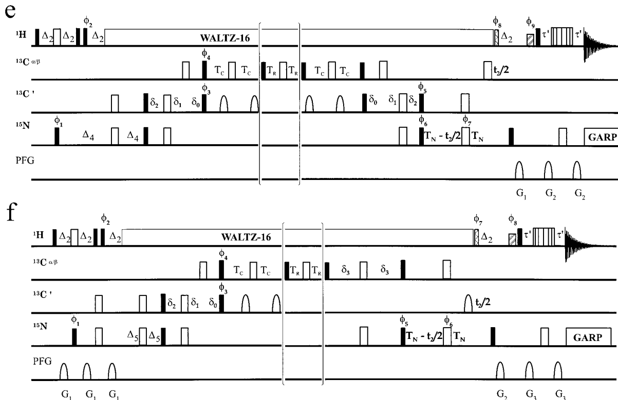
FIG. 3. Pulse sequences of the new amino acid type-selective ^1\text{H} - ^{15}\text{N} correlations. The pulse sequences yield spectra for Gly (a and c), Ala, Thr, Ile, and Val (b and d), and Asn and Gln (e and f). Pulses of 90^\circ and 180^\circ are represented by thin black filled and thick unfilled bars, respectively. The water-selective 90^\circ ^1\text{H} flip-back pulse is represented by a striped thick bar; a hatched thin bar stands for a 90^\circ flip-back ^1\text{H} pulse at the end of the ^1\text{H} -decoupling sequence. Magnetic field gradients as well as shaped 180^\circ ^{13}\text{CO} pulses are represented by sine shapes. Pulses applied at the ^{13}\text{C}^\alpha , ^{13}\text{C}^{\alpha/\beta} , or ^{13}\text{CO} resonance frequencies were adjusted to provide a null at the corresponding ^{13}\text{CO} or ^{13}\text{C}^\alpha frequencies. The square ^{13}\text{C}^\alpha 90^\circ and 180^\circ pulses were set to 54 and 48 \mu\text{s} , respectively. The square ^{13}\text{C}^{\alpha/\beta} 90^\circ and 180^\circ pulses were set to 49 and 44 \mu\text{s} , respectively. The square ^{13}\text{CO} 90^\circ and 180^\circ pulses were set to 54 and 108 \mu\text{s} , respectively. The shaped 180^\circ ^{13}\text{CO} was applied as G3 Gaussian cascade (50) with a duration of 256 \mu\text{s} . In the Thr/Ala experiments (b) and (d) the striped thick bar with an asterisk stands for a band-selective 180^\circ REBURP pulse (51) at 68.5 ppm with a duration of 1024 \mu\text{s} , while this pulse was applied as a normal square 180^\circ pulse in all the other experiments. Unless indicated otherwise, pulses are applied with phase x . Proton hard pulses were applied with 25 kHz field strength; WALTZ-16 (52) of ^1\text{H} spins was achieved using a field strength of 3.1 kHz. The same field strength was used for the subsequent 90^\circ flip-back ^1\text{H} pulse. The water-selective 90^\circ square pulse had a duration of 1 ms. GARP-1 decoupling (53) of ^{15}\text{N} was achieved using a field strength of 830 Hz. Water suppression was obtained using WATERGATE implemented with a 3–9–19 pulse (54). The gradients were applied as a sinusoidal function from 0 to \pi . The carrier frequencies were centered at ^1\text{H} = 4.8 ppm, ^{15}\text{N} = 119.6 ppm, ^{13}\text{C}^\alpha = 55 ppm, ^{13}\text{C}^{\alpha/\beta} = 45 ppm, and ^{13}\text{CO} = 175 ppm. The following delays were used: \Delta_1 = 3.5 ms, \Delta_2 = 5.5 ms, \Delta_3 = 7.0 ms, \Delta_4 = 13.5 ms, \Delta_5 = 8.0 ms, \delta_0 = 4.5 ms, \delta_1 = 6.9 ms, \delta_2 = 11.4 ms, \delta_3 = 9.3 ms, T_N = 11 ms, \tau' = 2.25 ms, T_R = 4.5 ms (except for the TAVI-experiments where T_R = 3.7 ms), T_C = 4.5 ms. To achieve quadrature detection in the indirect dimension the States-TPPI-States protocol (55) was used in all experiments. All spectra were processed using XWINNMR (Bruker AG). (a) G-( i + 1 )-HSQC. The phase cycling was: \phi_1 = 16 ( x ), 16 ( -x ); \phi_2 = 2 ( 45^\circ ), 2 ( 135^\circ ), 2 ( 225^\circ ), 2 ( 315^\circ ); \phi_3 = x, -x ; \phi_4 = 50^\circ ; \phi_5 = x ; \phi_6 = 8 ( x ), 8 ( y ), 8 ( -x ), 8 ( -y ); \phi_7 = -y ; \phi_8 = -x ; \phi_{\text{rec}} = 2 ( x , 2 ( -x ), 4 ( -x , 2 x , -x ), 2 ( x , 2 ( -x ), x )). States-TPPI phase cycling was applied to phase \phi_5 . Gradients had the following duration and strength: G_1 = 800 \mu\text{s} (7 G/cm), G_2 = 900 \mu\text{s} (28 G/cm), G_3 = 1 ms (21 G/cm). (b) A-( i + 1 )-HSQC (omitting the part in parentheses), TAVI-( i + 1 )-HSQC (including the part in parentheses and using a normal ^{13}\text{C}^{\alpha/\beta} 180^\circ pulse (*)), and TA-( i + 1 )-HSQC (including the part in parentheses and using a Thr- \text{C}^\beta -selective 180^\circ REBURP pulse (*) at 68.5 ppm). The phase cycling was: \phi_1 = 24 ( x ), 24 ( -x ); \phi_2 = 2 ( 30^\circ ), 2 ( 90^\circ ), 2 ( 150^\circ ), 2 ( 210^\circ ), 2 ( 270^\circ ), 2 ( 330^\circ ); \phi_3 = x, -x ; \phi_4 = 50^\circ ; \phi_5 = x ; \phi_6 = 12 ( x ), 12 ( y ), 12 ( -x ), 12 ( -y ); \phi_7 = -y ; \phi_8 = -x ; \phi_{\text{rec}} = 3 ( x , 2 ( -x ), x ), 6 ( -x , 2 ( x ), -x ), 3 ( x , 2 ( -x ), x )). States-TPPI phase cycling was applied to phase \phi_5 . The gradients had the following duration and strength: G_1 = 800 \mu\text{s} (7 G/cm), G_2 = 800 \mu\text{s} (28 G/cm), G_3 = 1 ms (21 G/cm). (c) G-( i, i + 1 )-HSQC. The phase cycling was: \phi_1 = x, -x ; \phi_2 = 2 ( 45^\circ ), 2 ( 135^\circ ), 2 ( 225^\circ ), 2 ( 315^\circ ); \phi_3 = 8 ( x ), 8 ( -x ); \phi_4 = 4 ( x ), 4 ( y ), 4 ( -x ), 4 ( -y ); \phi_5 = 4 ( -y ), 4 ( y ); \phi_6 = (-x) ; \phi_{\text{rec}} = x , 2 ( -x ), x , 2 ( -x , 2 ( x ), -x ), x , 2 ( -x ), x ). States-TPPI phase cycling was applied to phase \phi_5 . The gradients had the following duration and strength: G_1 = 1 ms (7 G/cm), G_2 = 800 \mu\text{s} (28 G/cm), G_3 = 1 ms (21 G/cm). (d) A-( i, i + 1 )-HSQC (omitting the part in parentheses), TAVI-( i, i + 1 ) (including the part in parentheses and using a normal ^{13}\text{C}^{\alpha/\beta} 180^\circ pulse (*)), and TA-( i, i + 1 )-HSQC (with the part in parentheses and a Thr- \text{C}^\beta -selective 180^\circ REBURP pulse (*) at 68.5 ppm). The phase cycling was: \phi_1 = 24 ( x ), 24 ( -x ); \phi_2 = 2 ( 30^\circ ), 2 ( 90^\circ ), 2 ( 150^\circ ), 2 ( 210^\circ ), 2 ( 270^\circ ), 2 ( 330^\circ ); \phi_3 = x, -x ; \phi_4 = 12 ( x ), 12 ( y ), 12 ( -x ), 12 ( -y ); \phi_5 = -y ; \phi_6 = -x ; \phi_{\text{rec}} = 3 ( x , 2 ( -x ), x ), 6 ( -x , 2 ( x ), -x ), 3 ( x , 2 ( -x ), x )). States-TPPI phase cycling was applied to phase \phi_5 . The gradients had the following duration and strength: G_1 = 800 \mu\text{s} (7 G/cm), G_2 = 800 \mu\text{s} (28 G/cm), G_3 = 1 ms (21 G/cm). (e) N-( i + 1 )-HSQC (omitting the part in parentheses) and QN-( i + 1 )-HSQC (including the part in parentheses). The phase cycling was as follows: \phi_1 = 16 ( x ), 16 ( -x ); \phi_2 = 2 ( 45^\circ ), 2 ( 135^\circ ), 2 ( 225^\circ ), 2 ( 315^\circ ); \phi_3 = 310^\circ , \phi_4 = 32 ( x ), 32 ( -x ); \phi_5 = 50^\circ ; \phi_6 = x, -x ; \phi_7 = 8 ( x ), 8 ( y ), 8 ( -x ), 8 ( -y ); \phi_8 = 4 ( -y ), 4 ( y ); \phi_9 = -x ; \phi_{\text{rec}} = 2 ( x , 2 ( -x ), x ), 4 ( -x , 2 ( x ), -x ), 2 ( x , 2 ( -x ), x ), 2 ( -x , 2 ( x ), -x ), 4 ( x , 2 ( -x ), x ), 2 ( -x , 2 ( x ), -x )). States-TPPI phase cycling was applied to phase \phi_6 . The
